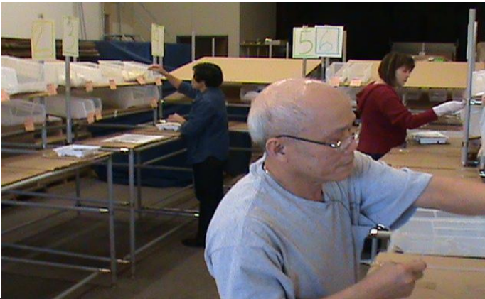
The STI lean team tested single-piece flow in a basic simulation of a U-shaped cell, top. Later, team members checked walk paths in a more complex simulation, bottom.
