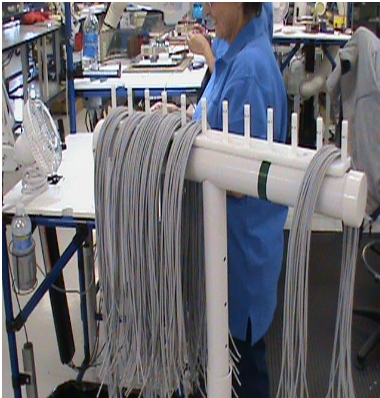
A heijunka post loaded by the team leader levels production through the cell. Each section is an hour's worth of work.
