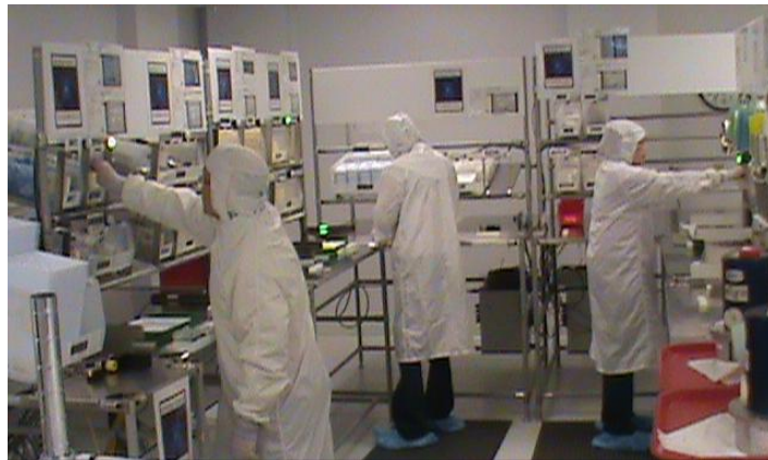
After: The Do phase at STI transformed clean room kit assembly from batch to a single piece flow cell with three walk paths.
