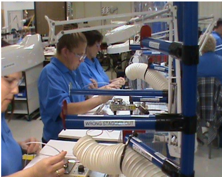
Cell operators drape any defects on horizontal posts that are labeled by type.
